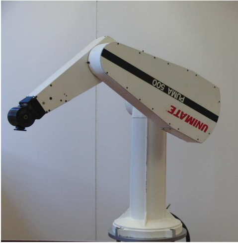
Fig. 18. The classic Puma 560 arm is a chain of three rotatable bodies (excluding the end effector) attached to a rigid base. This yields a three-dimensional C-space, which is handled by the standard planning algorithms. (Photo courtesy of the Technical University of Berlin.)
